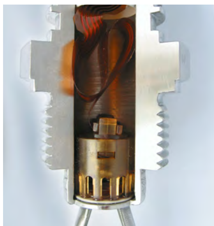
Bimorph or stack drive, the heart of the Endress+Hauser vibronic point level switch
